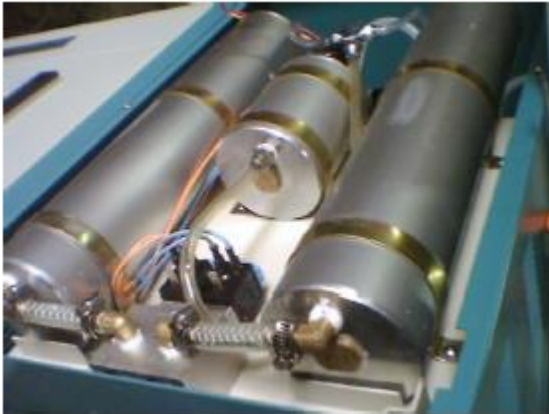
Figure nº 1.8 – Pressure Swing Adsorption (oxygen generator in model CAS+® 10)
